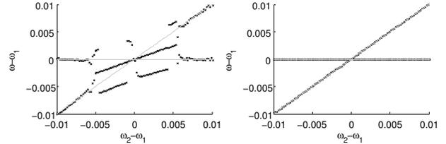
**Fig. 4.** Frequency estimations for two partials with close frequencies, 100 signals, no noise, 50 samples per signal. left: SOMP, right: nonuniform multichannel MUSIC
